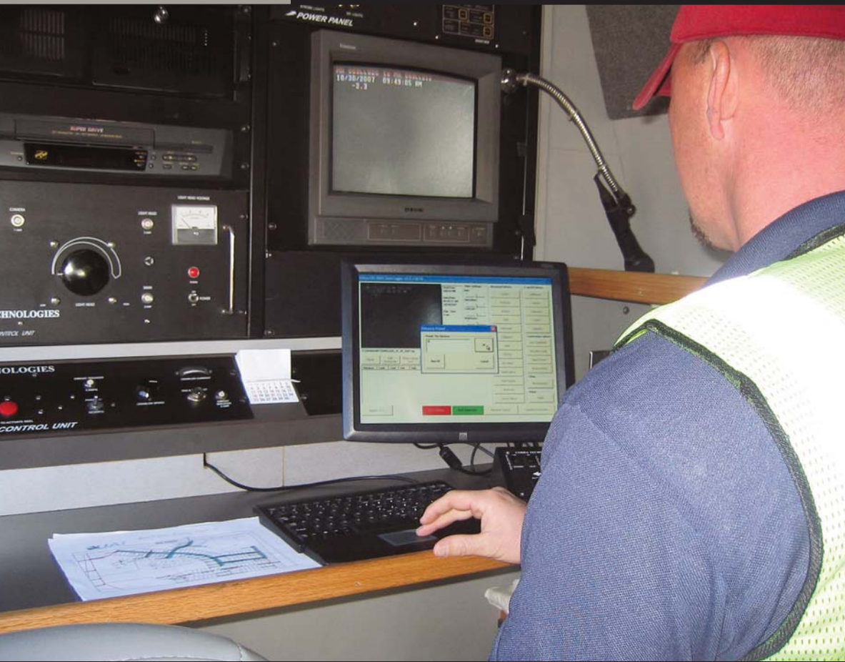
Murfreesboro rehabilitation technician Ashley Hopkins enters pipe inspection data into the computer. Hard-drive data storage greatly enhances the city's inspection program. (Photo courtesy of Murfreesboro Water & Sewer Department)
